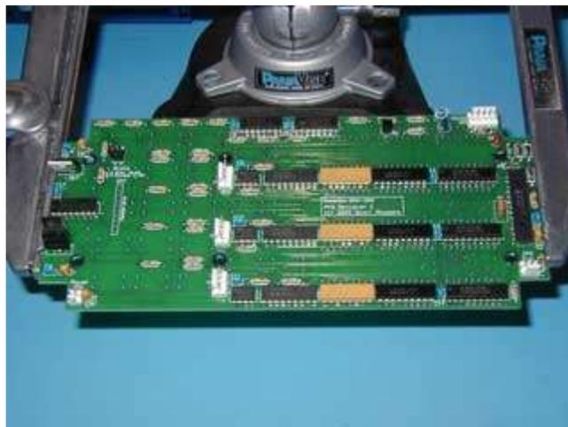
Install the ICs next but be careful not to force them into the PCB. If the pins do not line up, gently bend them by pressing the side of the IC on a hard surface with a static safe bag between the pins and the surface. If completing the build in stages, first fit U2, U7,8 & 9 and resistor pack R12, followed by displays DS1,2 and 3 (the top row of displays).
