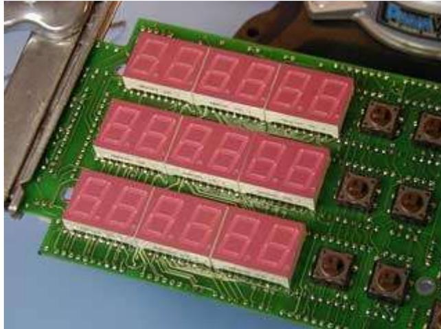
At this point, the first line of the display can be tested, and should display dro350. If not, then fault finding at this stage is easier than with a fully populated board. Contact the user group for help.
