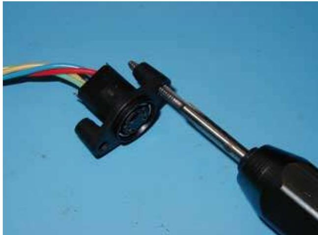
*Tap the Mini-Din Scale Connectors with an M2.5*
