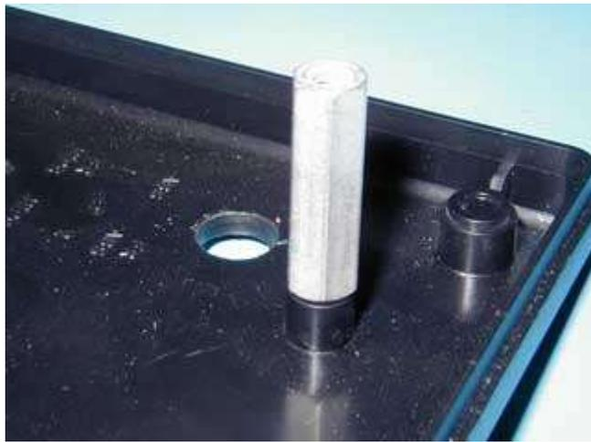
*Hex Stand off Installed in the Back Panel ( Replace with UK picture when available )*
