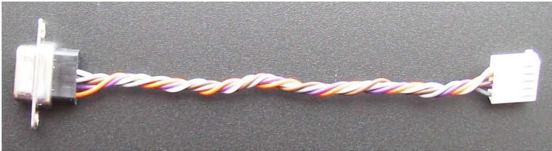
*Programming Cable DB-9 Serial Connectors*
