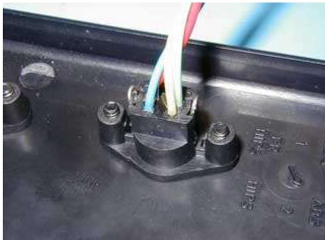
*Scale Connector Mounted to Back Panel with M2.5 Screws*
