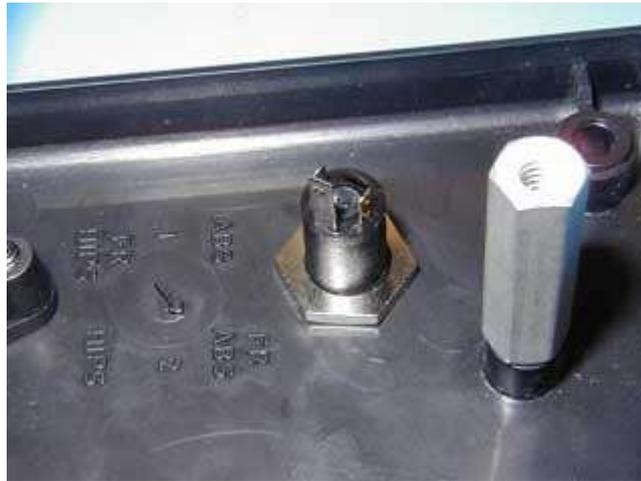
*Auxiliary Connector Mounted to the Back Panel with the Included Nut
