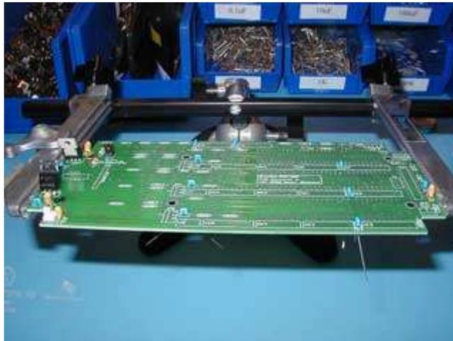
Before installing any ICs, it is easiest to install the decoupling capacitors first. All the decoupling capacitors are 0.1 $\mu$ F ceramics and do NOT have polarity so you can solder them in any orientation. The decoupling capacitors have designators C2, C8, C9, C10, C11, C12, C13, C14, C16, and C17.
