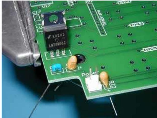
The 5 volt power supply consists of device U16 and capacitors C3, C4, and C15. An optional MTA-100 connector can also be used for the power entry connector JP6. Pay special attention paid to the polarity of C15 and C3. These are tantalum capacitors and have a marking on the POSITIVE lead. Make sure to insert the marked lead to the side marked with a + on the PCB. Also notice that the pad this lead is inserted into is square instead of round.
