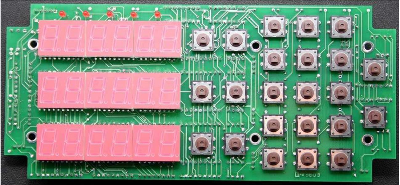
*Display Side of a Completed DRO-350 PCB*
