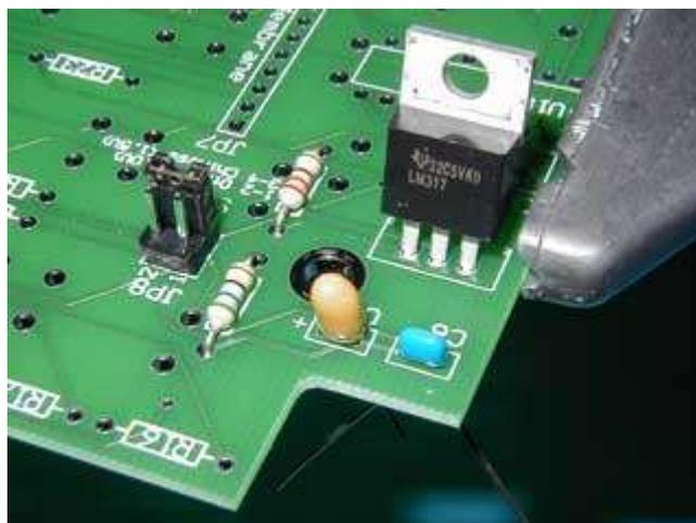
The 1.5 volt power supply is what powers the Chinese scales and consists of device U17, capacitors
