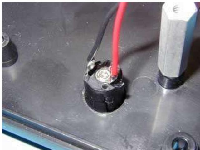
*DC Power Connector Pushed Through the Hole in the Back Panel
