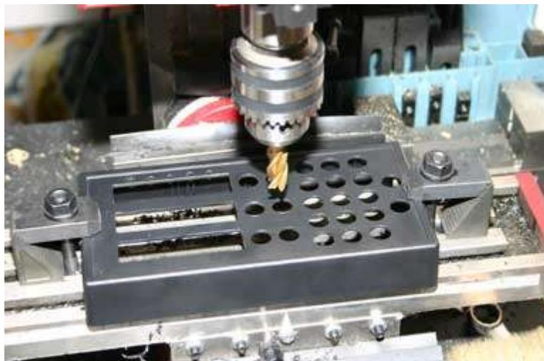
*DRO-350 Front Panel After Milling and Drilling Operations*
