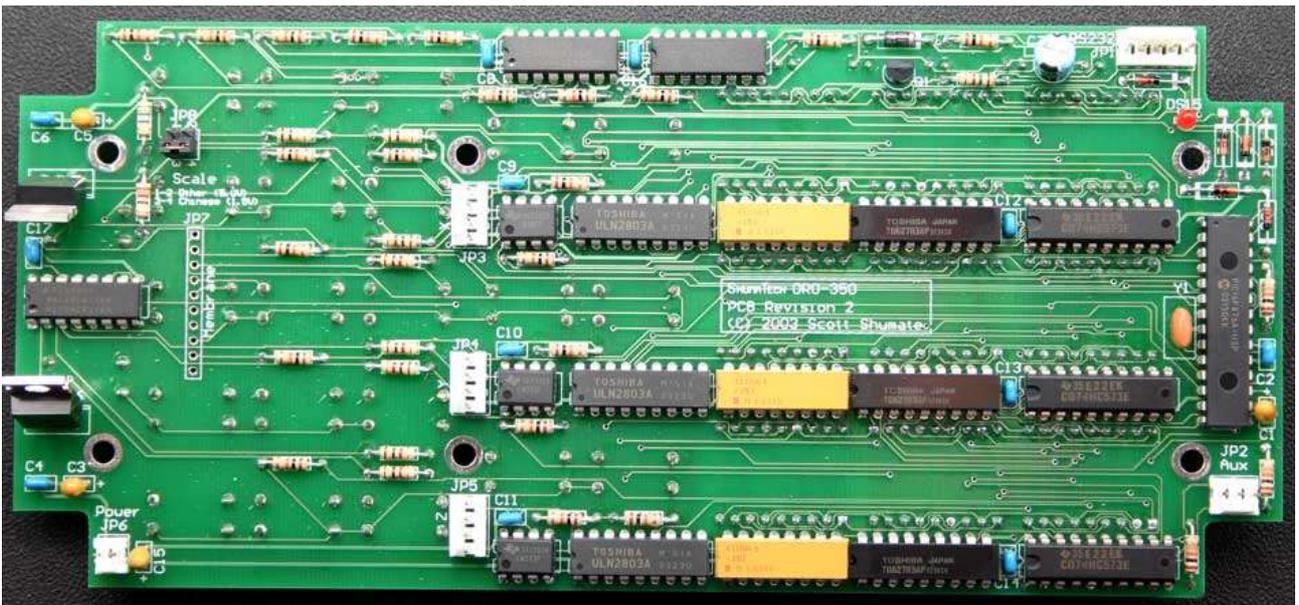
*Component Side of a Completed DRO-350 PCB*
