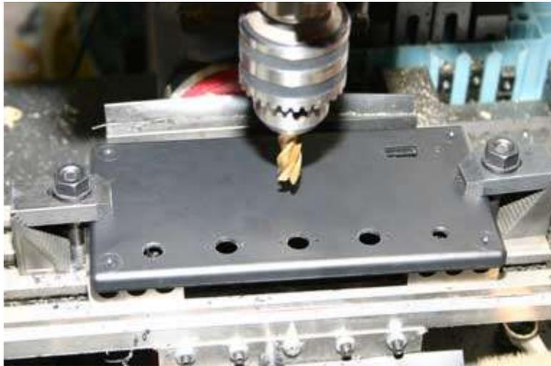
*DRO-350 Rear Panel After Milling and Drilling Operations*
