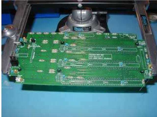
Next, install all of the resistors. It is easiest to use a triangular [lead forming tool](#) but not required. The resistor lead are spaced at 400 mil. Run through the BOM installing each resistor value at its correct designator. It is easiest to solder the resistors from the component side. After soldering, you probably want to run back through the BOM double checking the correct resistor values.
