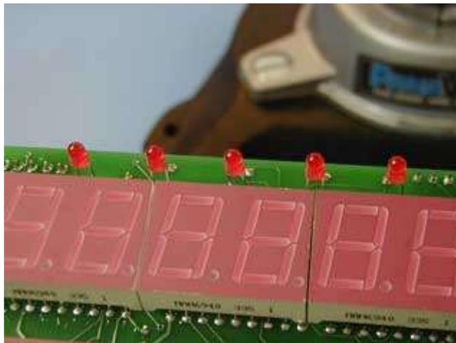
There are five T1-size (3mm) LEDs on the display side of the PCB. The LEDs have designators DS10-DS14 on the schematic but note that there is no silkscreen on the display side of the PCB. The pads are easy to locate since they are just above the seven segment displays and are the only pads without something soldered in them.
